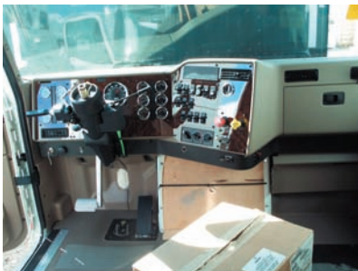
Complete trim of day and sleeper cabs, including all dash and driver control modules, window regulators, bunk/interior and exterior trim, glass and all wiring.
