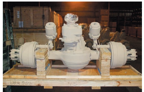
Commercial and Military front and rear axles. Assemble brake groups, sensors, bearings, seals, disk and drum brakes, yokes, CARC painting and axle shafts.
