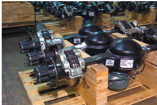
Commercial and Military front and rear axles. Assemble brake groups, sensors, bearings, seals, disk and drum brakes, yokes, CARC painting and axle shafts.
