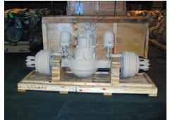
drained, set in a water vapor bag with 2 desiccant bags, sealed with a humidity indicator and crated with an inspection port on the side of the crate. These preservation methods are required by the contract in the supplementary instruction portion and defined in Mil Std 2073. Rollins was one of the first suppliers to assist the Prime in their efforts to provide MRAP Service Parts. Both Rollins
